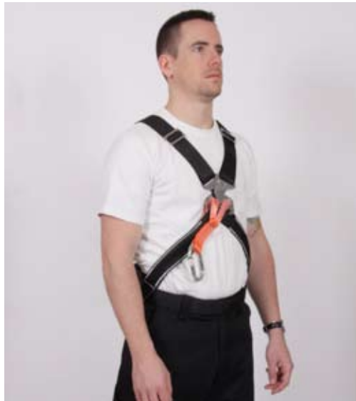
14. How finished fitted harness should appear
